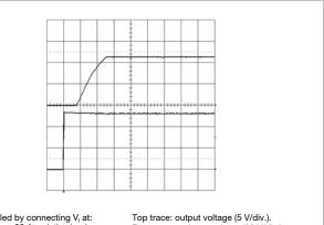
Start-up enabled by connecting  $V_l$  at:  $T_{ref}$  = +25°C,  $I_0$  = 33 A resistive load,  $V_l$  = 53V.
