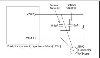
Output ripple and noise test setup
