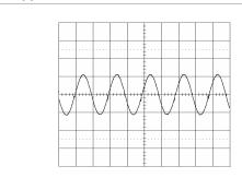
Output voltage ripple at:  $T_{ref} = +25^{\circ}C$ ,  $V_{l} = 53$  V,  $l_{O} = 33$  A resistive load.
