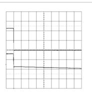
Shut-down enabled by disconnecting V $_{\rm I}$  at:  $T_{\rm ref}=+25^{\circ}C,\,I_{O}=33$  A resistive load, V $_{\rm I}=53$  V.
