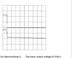
Shut-down enabled by disconnecting V $_{\rm I}$  at:  $T_{\rm ref}=+25^{\circ}C,~I_{O}=25$  A resistive load, V $_{\rm I}=53$  V.
