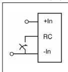
The products are fitted with a remote control function referenced to the primary negative input connection (- In), and positive logic options available. The RC function allows the DC/DC converter to be turned on/off by an external device like a semiconductor or mechanical switch. The RC pin has an internal pull up resistor to + In.
