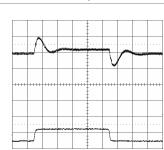
Output voltage response to load current step-change (8.25-24.75-8.25 A) at:  $T_{\text{ref}}$ =+25°C,  $V_{\text{I}}$  = 53 V.
