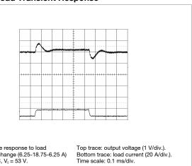
Output voltage response to load current step-change (6.25–18.75–6.25 A) at:  $T_{\rm ref}$ =+25°C,  $V_{\rm l}$  = 53 V.
