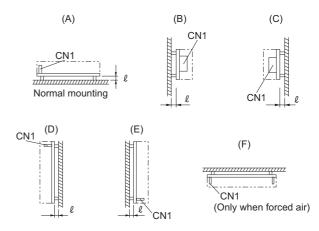
■In case of metal chassis, keep more than 8mm for the part of ℓ to insulate between lead of component and metal chassis. If it is less than 8mm, insert the insulation sheet between power supply and metal chassis.
