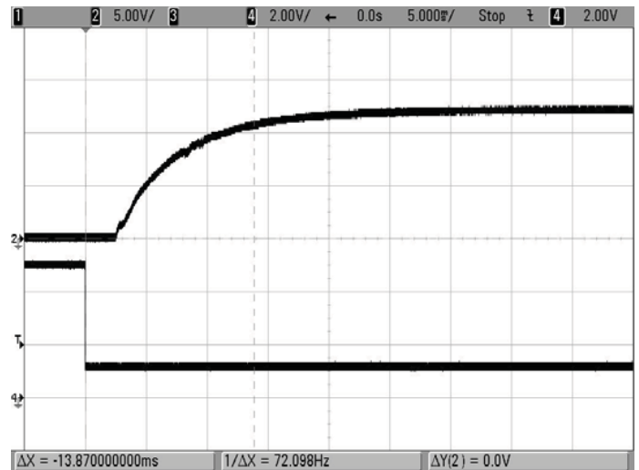
Enable Start-up (Vin=48V, Iout=5A, Load=1000µF Ta=+25°C) Trace 2=Output, Trace 4= Enable.
