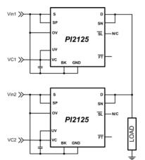
Figure 1: Pl2125 High Side Active ORing
