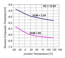
**Figure 8:** Reverse comparator threshold vs. temperature. **VCM:** Common Mode Voltage
