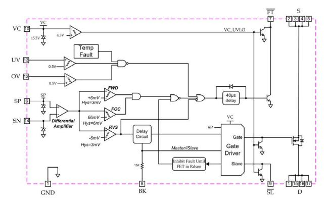
Figure 3: Pl2125 Internal Block Diagram
