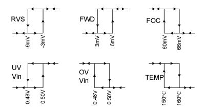
Figure 4: Comparator hysteresis, values are for reference only. Please refer to the electrical specifications.
