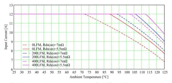
Figure 17: PI2125 input current de-rating based on maximum T<sub>J</sub>=150°C vs. ambient temperature
