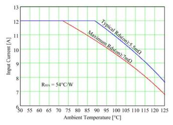
**Figure 2:** Pl2125 input current de-rating based on maximum T<sub>J</sub>=150°C vs. ambient temperature.
