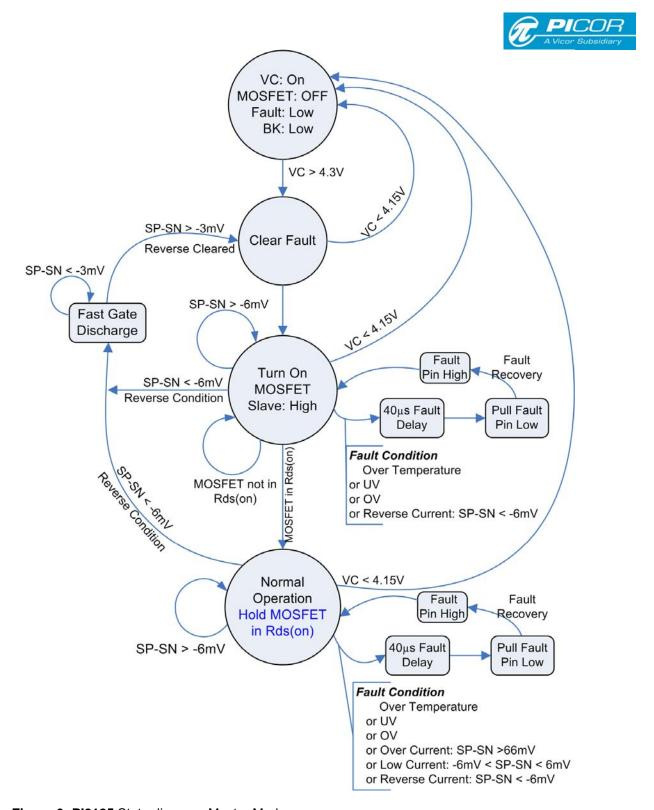
Figure 6: Pl2125 State diagram, Master Mode
