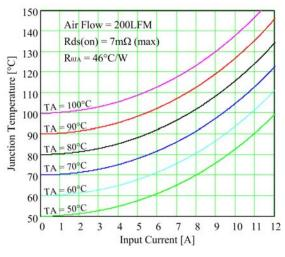
**Figure 14:** Junction Temperature vs. Input Current (200LFM)
