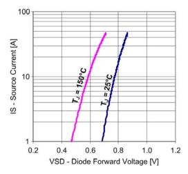
Figure 12: Internal MOSFET source to drain diode forward voltage (pulsed ≤ 300μs)
