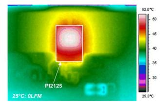
**Figure 15:** PI2125 mounted on PI2125-EVAL Thermal Image picture, Iout=12A, T<sub>A</sub>=25°C, Air Flow=0LFM
