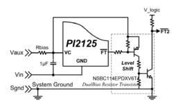
Figure 19: FT Level shift circuit
