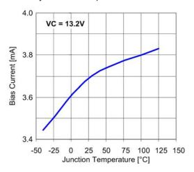
Figure 9: Controller bias current vs. temperature
