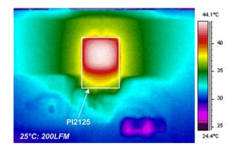
**Figure 16:** PI2125 mounted on PI2125-EVAL
