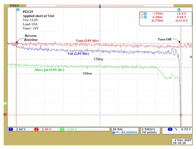
Figure 18: Plot of PI2125 response time to reverse current detection (Example 1, Figure 23)
