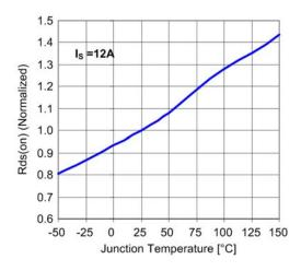
**Figure 11:** Internal MOSFET on-state resistance vs. temperature
