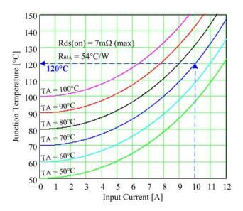
Figure 22: Example 1 final junction temperature at  $10A/70^{\circ}C$  T<sub>A</sub>
