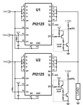
Figure 23: Pl2125, 12V floating Active ORing application
